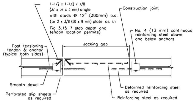
Fig. 3.16—Typical doweled joint detail for post-tensioned slab.
