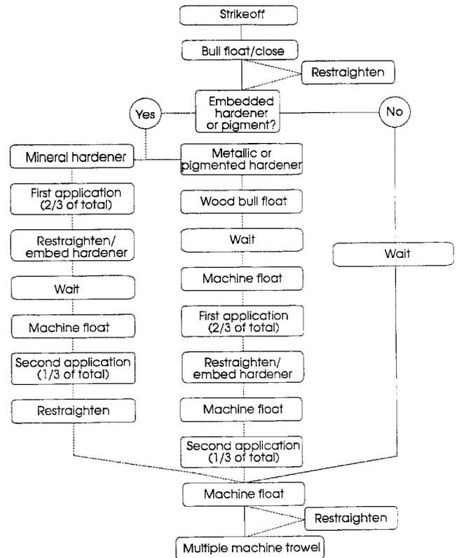
NOTE: Dashed lines indicate optional procedures that may be included as a part of the finishing operation. Restraightening is encouraged as a means of improving surface flatness.
