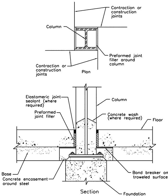
Fig. 3.4—Typical isolation joint at wide flange column.
