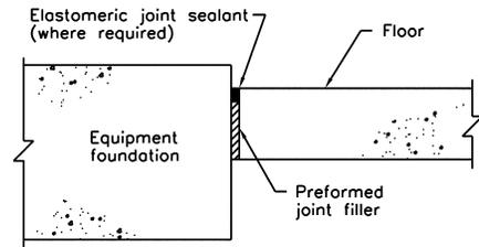
Fig. 3.5—Typical isolation joint around an equipment foundation.
